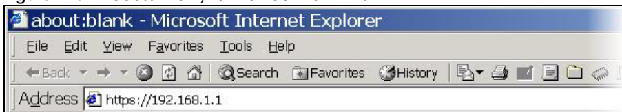
Figure 715 Access the Zyxel Device Via HTTPS
